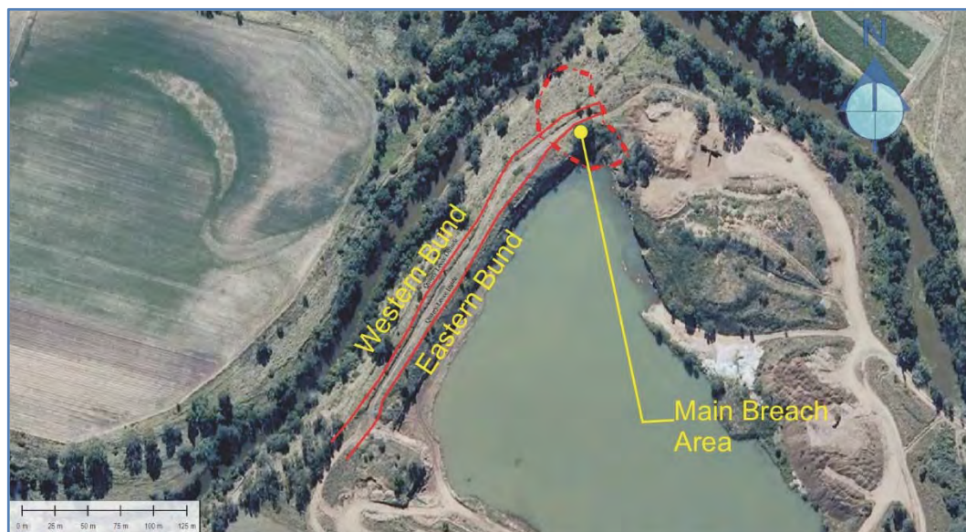
Figure 4.3: Image showing location of pre-flood bunds and the location of the main breach
