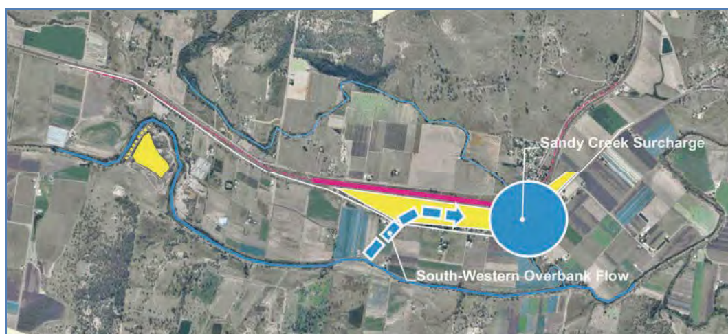
Figure C12: Simplified flooding locality, south-western overbank inundation.
