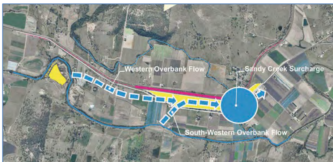
Figure C13: Simplified flooding locality, western overbank inundation.
