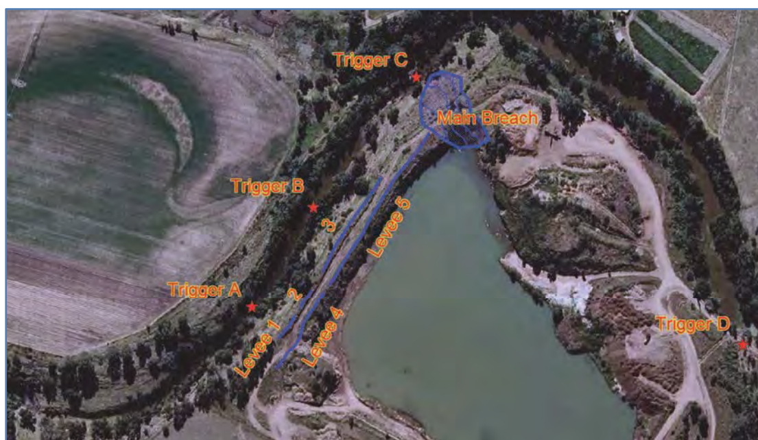
Figure C10 – Quarry failure trigger level locations
