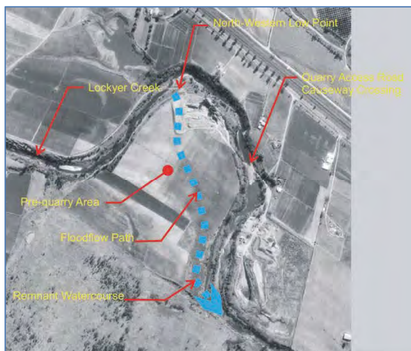
Figure C23: Quarry area in 1982 overlaid with flood path
